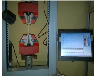
Figure 2: Bamboo splint in tension
