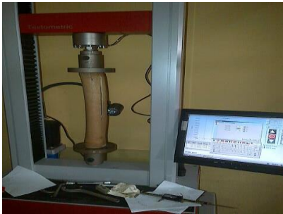
Figure 1: Bamboo culm in compression
