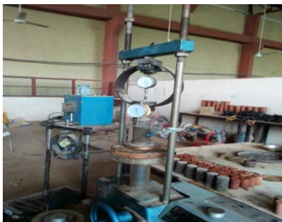
Fig. 1: Unconfined compressive strength test
