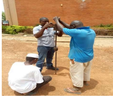
Fig. 11: DCP Test on a compacted surface
