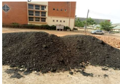
Fig. 2: Pile of milled RAP
