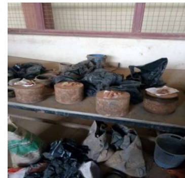
Fig. 4: Compacted samples for CBR test
