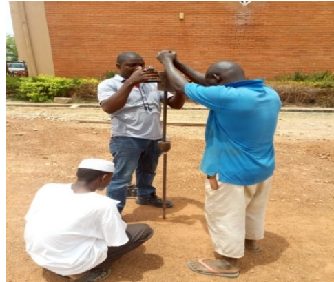
Fig. 11: DCP Test on a compacted surface
