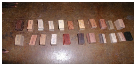
Fig. 1. Test Samples of Some Nigerian Timber
