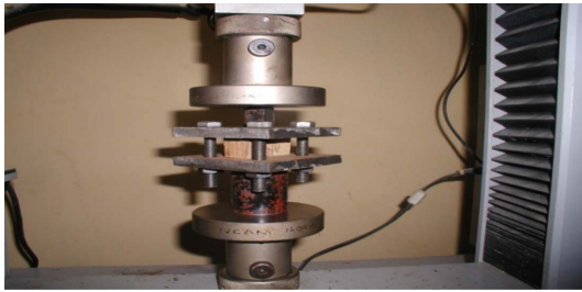
Fig. 6. Test Set-up for Shear Parallel to the Grain
