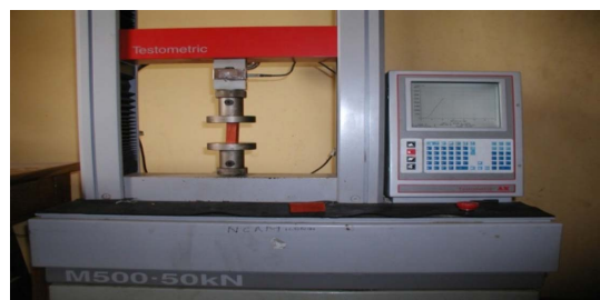
Fig. 4. Testing Set-up for Compression Parallel to the Grain
