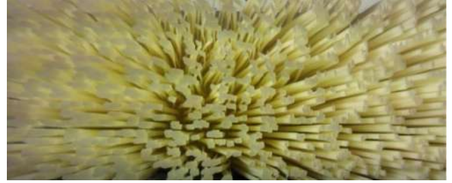
Fig. 2. A sectional plan view of the dense vegetation ( \phi = 0.1214 array).
