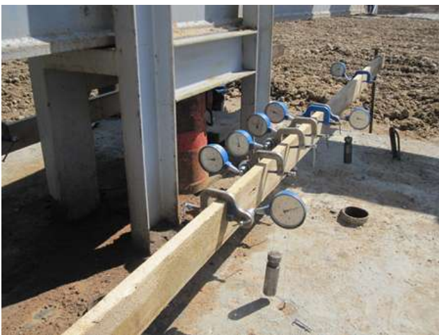
Fig. 2 Dial gauges Connected for Settlement Reading
