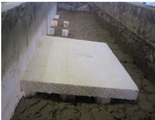
Figure-3: Modeled test piles prepared for loading
