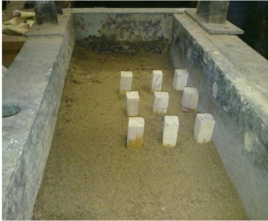
Figure 3: Modeled Test Piles Bored into the Soil
