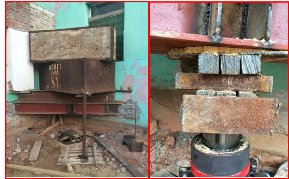
Figure 6: Load Test Modeled Test Piles
