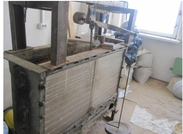
Figure 1. Testing tank and load application on soft clay
