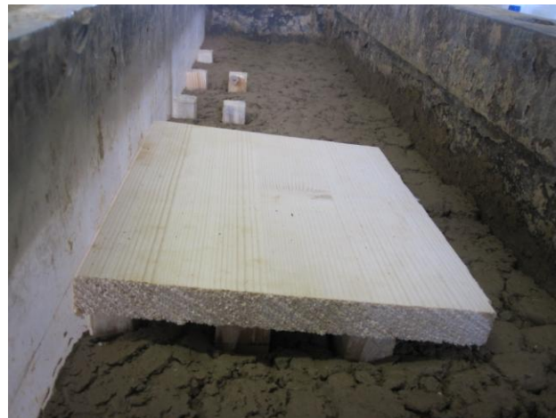
Figure 2. Testing tank and load application on soft clay
