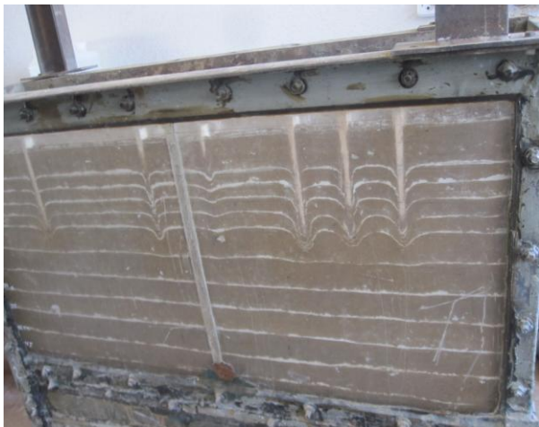
Figure 8. Testing Tank showing eaves, depression and settlement of piles
