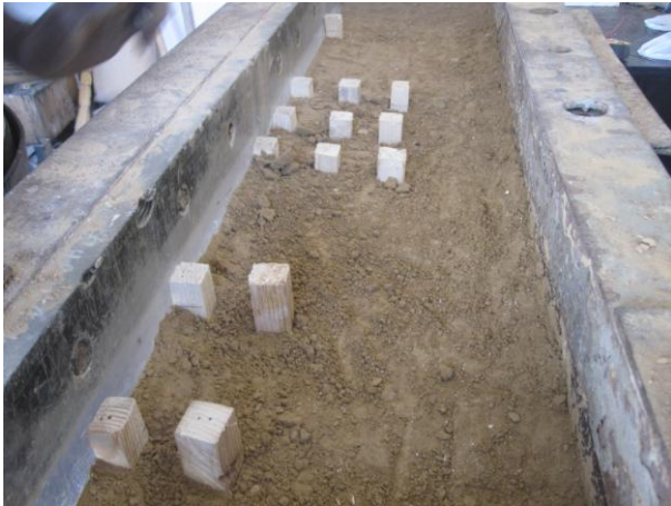
Figure 2. Pile driven into Clay Soil in the Tank
