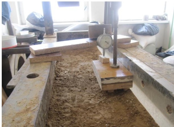
Figure 3. Settlement Measurement on Dial gauge
