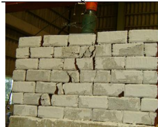
Figure 5 (a): Failure of a 2%MSWA stabilized wall.
