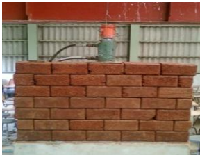
Figure 1: General arrangement of wall model for testing
