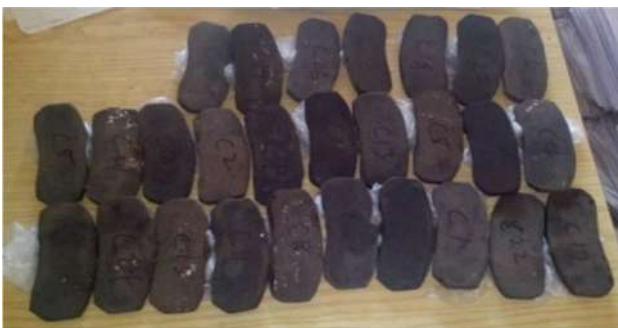
Fig. 2 Heat-treated coconut shell-reinforced brake pad samples
