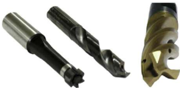
Fig. 3. Cutting tools for MQL (DGUV, 2010).
